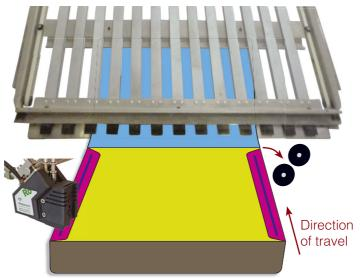
4 A Folding Plate is used to stop the inside panel travelling and force the two opposing sides downwards at the point of the main crease and marry them together through rollers.
