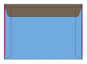
Additional process can then be applied in line such as Peel & Seal Tape as well as Red Stripper Tape to the Envelope Flap and then the flap can be folded close.
