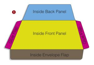
'Ploughs' are used on both Glue Flaps to turn them over ready for Glue to be applied. Sharp creases helps this process greatly.
